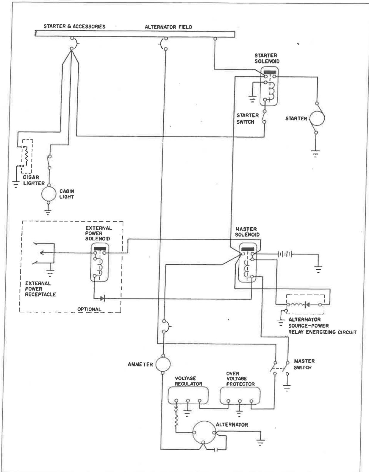
Alternator and Starter Schematic (Ser. nos. 7405001 through 7405290)
